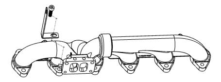
You now have the option to drill a hole through the OEM coolant pipe tab and secure the brackets using the together 1/4 bolt (1100110), 1/4" flat washer (1100111), 1/4" lock washer (1100112),and the 1/4" nut (1100113) supplied. Use a 5/16" drill bit to accomplish this.
