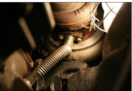
Disconnect the turbo oil supply and the turbo oil drain.
