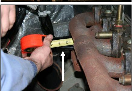
Remove the factory heat shield that covers the front of the manifold.
