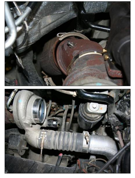
Disconnect the compressor outlet boot.
