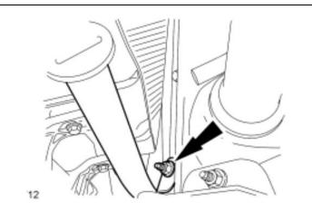
6. Remove the 2 passenger side exhaust manifold to turbocharger adapter pipe nuts.
