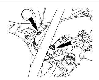
7. Remove the 8 bolts, 8 spacers and the passenger side exhaust manifold.
