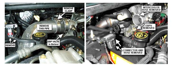
For ease of access and hook up, remove the connector from the EBP Valve and pull the wiring through and underneath to the front of the intake Y-plenum. This will allow access to install a Posi-Tap<sup>™</sup> or Connector harness.
