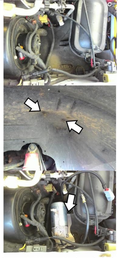
Install the supplied bolts and lock washers to attach the pump bracket to the fender where the vacuum pump previously attached. Reinstall the two 11mm nuts holding the vacuum reservoir.
