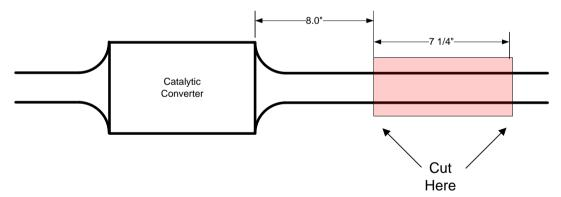
Remove any burrs from the ends of the cut pipes. Slide the supplied pipe adapters over each end of the cut pipes. Weld the adapter closest to the front of the vehicle in place. A good clean weld is needed to seal the high backpressure that the exhaust brake will create. The rear adapter will be secured with the supplied stainless band clamp.
