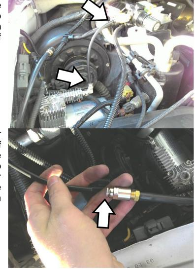
Install the intake air filter for the air compressor by adding a length of 1/4" air tubing to the rubber hose section. Then route this 1/4" line to a dry location (behind the regulator assembly is suggested). Install the "pancake" style filter supplied with the pump to the end of this tube.
