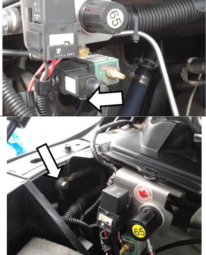
Connect the main power feed to the passenger side positive battery terminal clamp.
