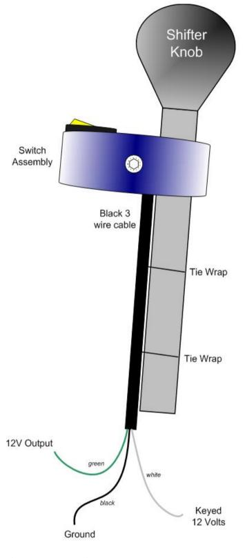
Locate one of the ignition switched power fuses in the fuse panel underneath the steering column. Traditionally this wire will be pink with a white tracer. Use a voltmeter to check the voltage of the wire. Use the supplied fuse tap to supply ignition switched power to the "Keyed 12 Volts" (white) wire of the rocker switch assembly.
