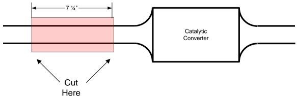
Clean off the cut ends of the intermediate pipe with a file to remove burrs left from cutting and then insert the adapter pipes onto each end of the now exposed pipes.
