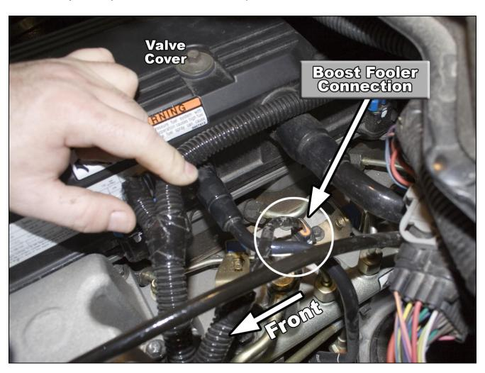
Unplug the factory boost connection from the engine. Plug the BD Boost Fooler inline with the factory plug, and then plug the remaining end of the BD Boost Fooler into the factory plug on the engine.
