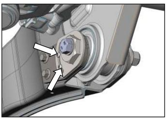
18. Adjust the adjustment cams so they are even on both sides and torque the lock plate bolts to 89 in/lbs. Then torque all radius arm (M18) mounting bolts to 222ft/lbs on DS/PS.
