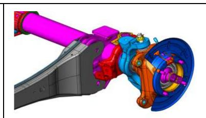
3. Remove the lower mounting bolts on the shock absorber from both sides of the vehicle. (18mm socket) then move the bottom of the shock out of the mount.
