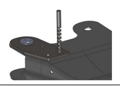
9. You can now remove the locating jig and enlarge the large hole with the supplied 1 3/8" hole saw.
