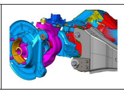
16. Now using two 2" box end wrenches rotate the adjustment cam until the bolt is at the most forward position on both DS/PS arms.
