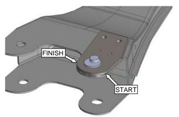
8. Using the plate to locate the hole positions drill the radius arm with the recommended 10.5mm drill bit or a 27/64" drill bit will do as well.
