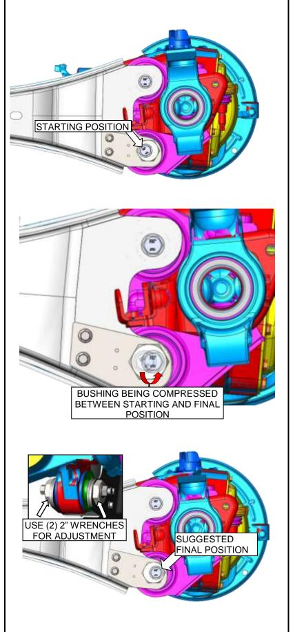
17. Install the lock plates (1302102) over the adjustment cams on each side of the arm and use the supplied lock plate bolts (1302106) to hold the plate down. Do both arms DS/PS and do not tighten completely.
