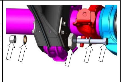
12. Install the rear factory mounting bolt do not completely tighten.
