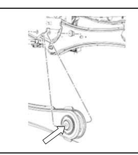
13. On the driver side remove the rear mounting bolt on the radius arm (24mm or 15/16" wrench). Then repeat the removal procedure following step 5.
