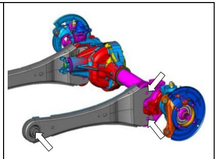
5. Removing the front two bolts on the passenger side radius arm, will release the arm from the vehicle.
