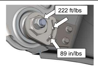
19. Reinstall the shock absorber lower bolt on the DS/PS and torque to 111 ft/lbs.
