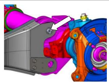
11. Install the supplied caster adjustors (1302101) into the lower connection using the supplied bolt (1302107), washers (1302110) and nut (1302109) do not completely tighten.
