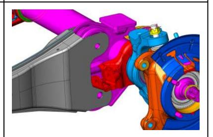
4. Loosen the three mounting bolts located on both radius arms and remove the rear mounting bolt on the passenger side radius arm. (24mm or 15/16" wrench)
