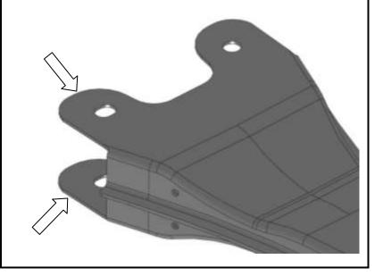
7. Insert the locating jig (1302105) into the radius arm and place the plate onto the locating jig, set the plate's position by ensuring the bottom edge of the plate is parallel with the edge of the radius arm & weld several 1/16" fillets x 1/4-1/2" long into place.
