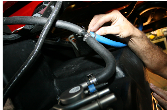
(Fig. 8) Attach “Y” to short primary vent line on sending unit and to tank’s front vent hose line. Hold with small gear clamps provided; make sure they are tight.
