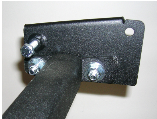
(Fig. 11) Shown: Right Hand Bracket for GM Cross Bar. The Cross Bar is held fast by tightening the 5/16” cap screw seen here at the upper left hand corner of the bracket. In severe applications it is recommended that the installer position the Cross Bar, mark the center of this cap screw hole, drill a hole in the front lip of the frame and then tighten the cap screw into the hole. It is advisable to apply Loctite Threadlocker or equivalent to the bolt. By early 2009, TITAN will be shipping a “Super Series” bracket with each tank as shown above. In a severe application, using this bracket, the installer may position the bracket, tighten down the cap screw as shown, and then drill a hole in the frame lip through the hole seen in the right hand corner of the bracket. An extra 5/16” cap screw and nylon locking nut are provided for fastening this extra hole.
