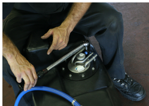
(Fig. 6) Tighten using torque wrench and a "star" pattern to ensure all nuts are equally tightened and the "O" ring gasket is properly seated.
