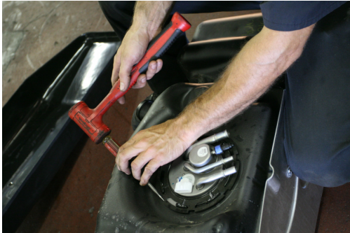
(Fig. 1) Remove sending unit from original equipment tank using mallet or hammer and large screwdriver.
