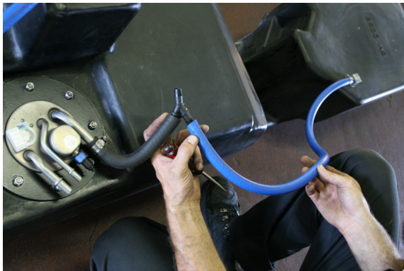
(Fig. 7) Replace cut-off portion of primary vent line onto sending unit. This figure illustrates how this part of the primary vent line, the “Y” and the tank’s front vent hose line will be connected when mounted in vehicle. The empty barb of the “Y” shown would be connected to primary vent line already attached to vehicle.
