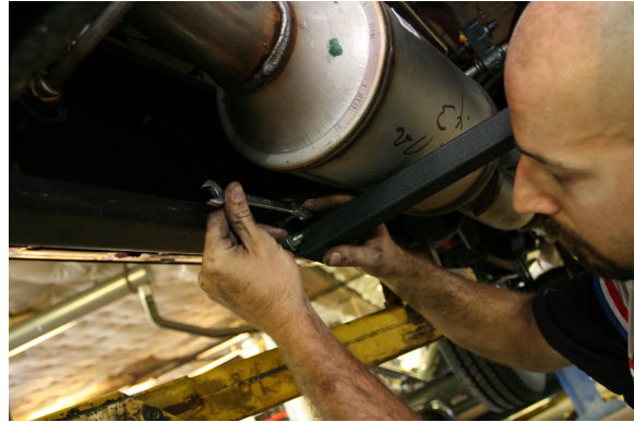
(Fig. 10) Tighten cross member against frame using 5/16” plated bolts, washers and nylon locking nuts provided. Note exhaust particulate filter above cross member.
