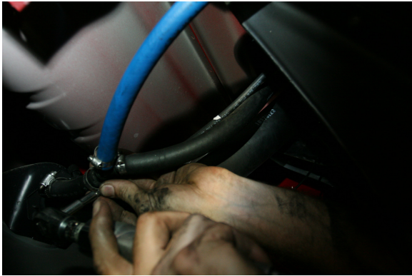
(Fig. 9) Cut primary vent line hose down approximately 8 inches from fill spout. Using second “Y” fitting provided, splice the two ends back together. Attach tank’s rear vent line to the remaining, third barb of the “Y”. Hold fast with small hose clamps provided; make sure they are tight.
