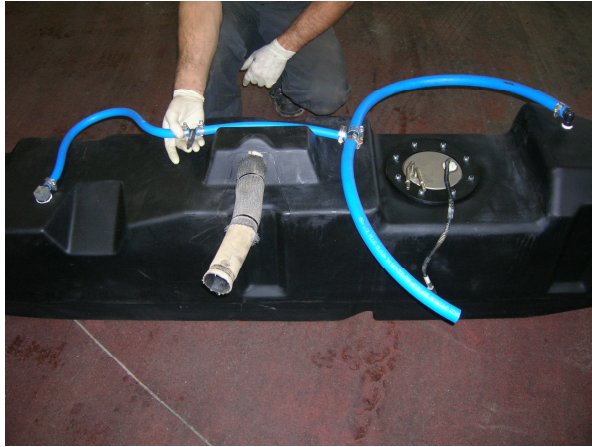
(Fig. 7) LONG BED tank vent hose arrangement. This photo shows how the 90° x 3/4" elbow and the front rollover valve are pointed at 45° angles toward each other and the inboard side of the tank. This is different than short bed plumbing. The technician's hand is holding the 1/2" x 1/2" x 1/4" tee with the check valve for the truck's 1/4" vent system (See Fig. 8). There is approximately 22" of 1/2" hose between the rollover valve and the tee. When the tank is lifted into the truck, the vent hoses may have to curve around and through the vehicle's cross members. Be sure there are no sagging hoses to trap fuel.
