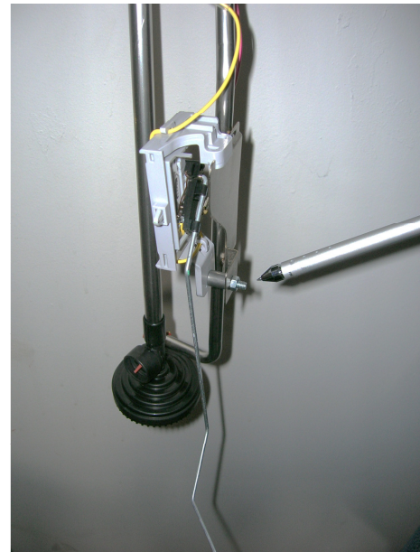
(Fig. 6) Level sensor has been removed and turned so as to face toward the rear of the truck when installed in the fuel tank. It is secured with pan-head screw, spacer (either steel or nylon) and nut. Pointer is indicating position of screw, nut and spacer.
