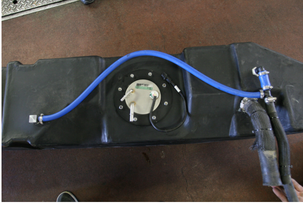
(Fig. 9) Top view of SHORT BED tank showing sending unit, tank vent hose plumbing, and original equipment fill hose and vent hose installation. The 1/2" x 1/2" x 1/4" tee is not shown installed in the 1/2" vent line hose. It will be installed approximately 2" from the rollover vent valve.
