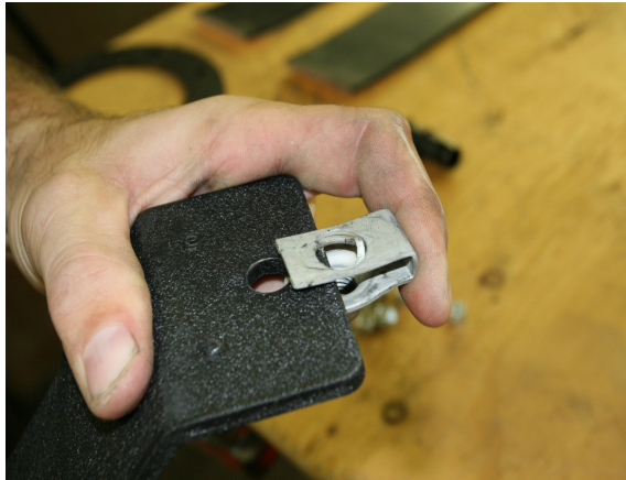
(Fig. 1) Remove threaded clip from original equipment tank's front strap and install on the Titan tank's front strap.
