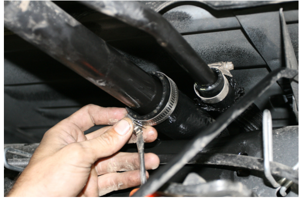
(Fig. 10) Attach fuel tank 1 1/2" fill hose and 3/4" vent hose to vehicle fill spout. Vent hose may have to be shortened about 6 inches to fit properly. On some long bed tanks, 1 1/2" fill hose may have to be extended with 3.35" hose extension.
