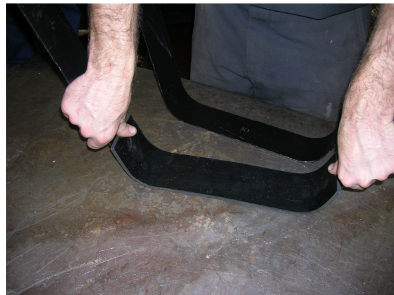
(Fig. 6) If TITAN™ Shield is NOT to be installed with the tank, then install Rubber Strap Bushings in tank mounting strap. Center the bushings in the bottom of the straps.
