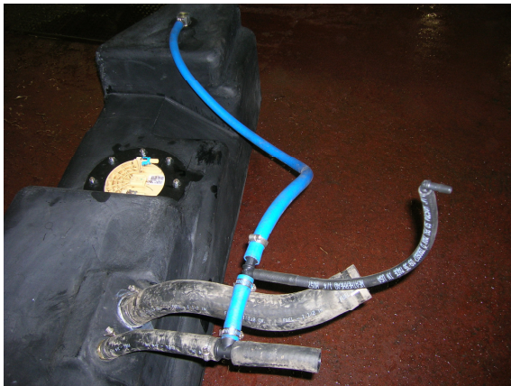
(Fig. 5) This shows final configuration for vent line system. Vent line on side of Vent Kit Assembly farthest from 3/4" OEM vent line should be left loose as it will not be connected permanently until tank is lifted into place and 1/2" vent line hose is threaded over the top of the truck frame.
