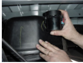
Step 3: Slide fuel valve from bracket.
