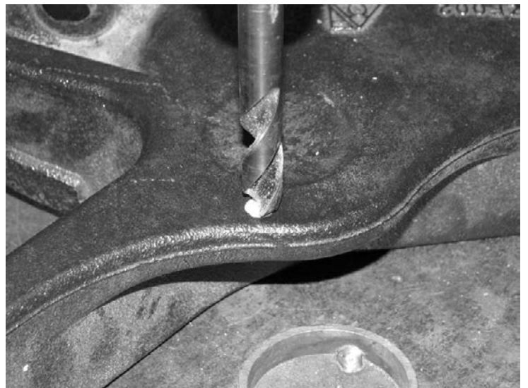
33. Remove the torsion bar bracket and drill a 1/2" hole. SEE PHOTO BELOW
