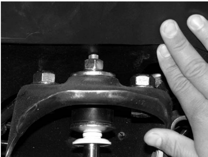
39. Install the lower mount of the shock into the rear shock mount on the torsion bar bracket that is mounted to the lower control arm. Use a 1/2"-13 x 2-3/4" bolt, washers and lock nut. Torque to 127 ft-lbs. SEE PHOTO BELOW
