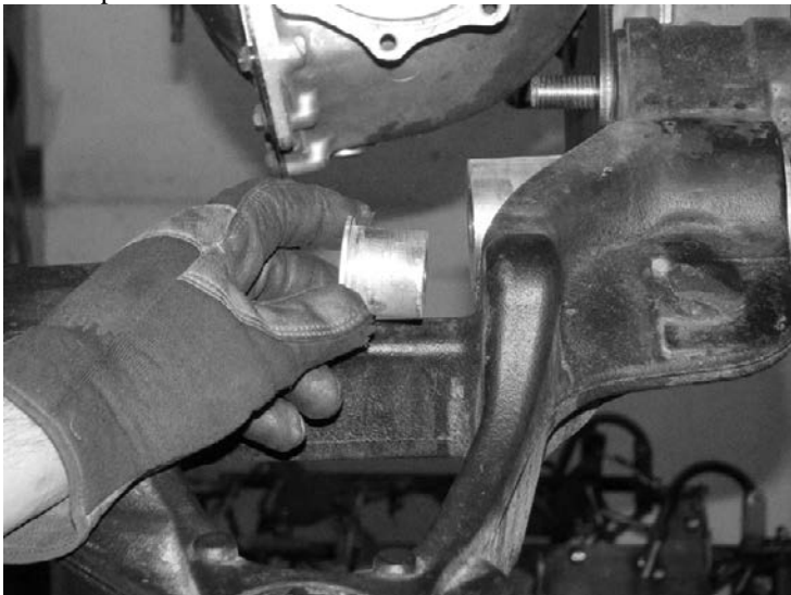
31. Locate the small aluminum RTS bushing (FT20481) and the lower control arm. Install the bushing into the front side of the shock mount where the OEM bushing was removed from in step 28. SEE PHOTO BELOW
