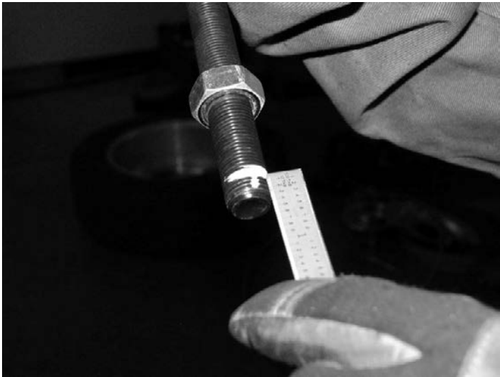
36. Remove 1/2" of thread from the tie rod using a die grinder. SEE PHOTO BELOW
