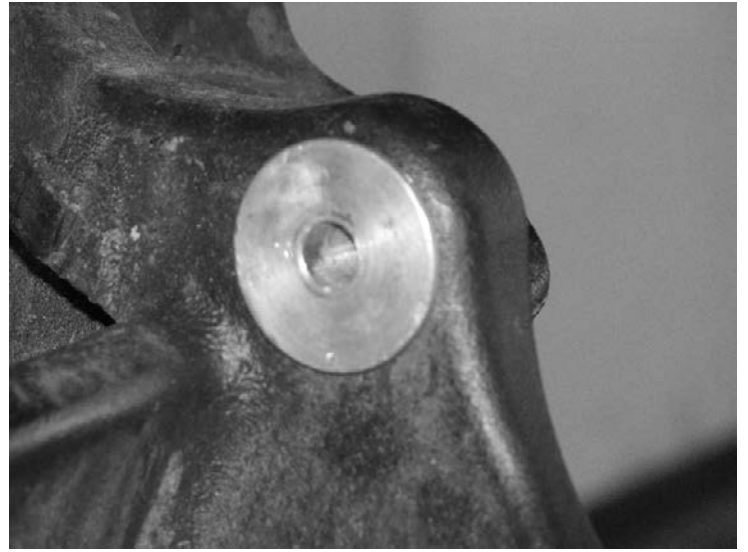
32. Locate the Torsion Bar mount for the Driver side lower control arm (FT20806). Temporarily install the torsion bar relocator to the arm by installing front and rear bolts. This will be done to mark a hole to be drilled that is needed to attach the bracket. Mark the hole using a transfer punch. SEE PHOTO BELOW
