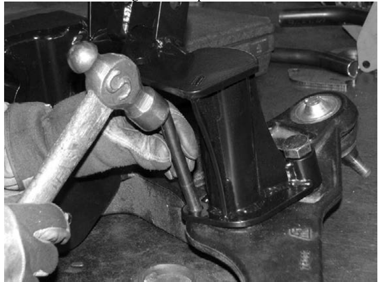
33. Remove the torsion bar bracket and drill a 1/2" hole. SEE PHOTO BELOW
