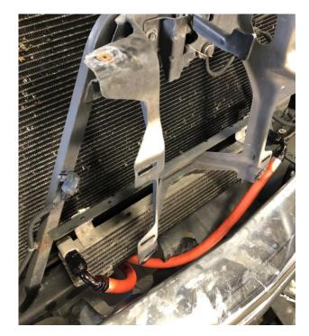
The medium length hose is routed from the transmission to the bottom-side radiator fitting. The 45 degree fitting is utilized on the radiator side, aligned slightly downward and toward the center of the chassis.
