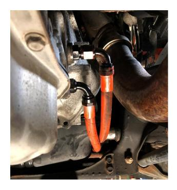
Route the lines uniformly along the left side of the chassis, just inside the frame rails by approximately 6-12".
