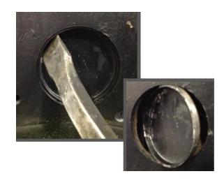
STEP 11: With the freeze plug removed, using a Scotch-Brite ™ pad and a degreasing solution, thoroughly clean the block surface area from the head down to the rear cover, as well as the bore where the freeze plug was previously installed. Be sure to remove any dirt or foreign debris.
