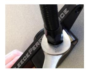
STEP 13: With assembly grease or light oil, lubricate the sealing O-ring on the coolant bypass thermostat housing (item 2), and pressit into place on the back of the engine block. The bypass coolant line should be oriented towards the passenger side of the vehide and over the exhaust manifold.
