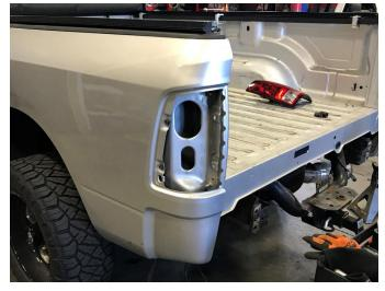
STEP 3: Remove the bolts that retain the bed of the truck to the frame. For the short bed model, there will be 6 fasteners. For the long bed model, there will be 8 fasteners.
