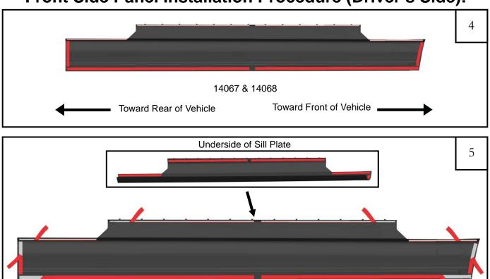
Peel back roughly 3" of red tape liner from the pieces of tape on the back side of the front part. Make sure red tape liner will be accessible when part is attached to truck.
