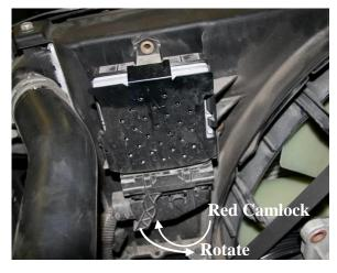
2. Unhook the TCM harness from the TCM by sliding the red camlock as shown and rotating the camlock lever. Gently pull the connector from the TCM.
