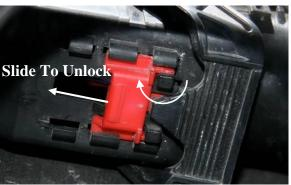
3. Remove the harness shroud from the TCM connector by gently prying the tabs and separating.
