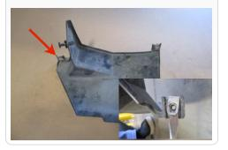
Attach the OE clip nut to the Fender liner bracket (J) as shown.
