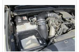
3. Loosen the 5 screws and remove the air box mounting tray. Retain the two rubber grommets to be used on the new scoop.
