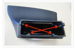
8. Install the Scoop Inlet assembly up into the Scoop Channel and secure using four 1/4-20x1.0" Screws (G) and 6mm washers (D). Tighten all the mounting hardware when you are satisfied with the position.
