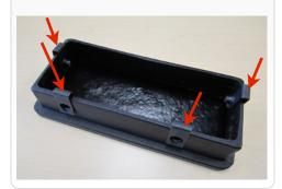
3. Install the Plug (C) into the Scoop Channel re-using the four 1/4-20 Screws (G) and Flat Washers (D).
