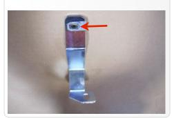
11. From outside the wheel liner, remove the screw attaching the plastic faring to the chrome bumper. Place the Fender liner bracket assembly behind the fender liner and attach using the OE screw.
