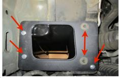
**6.** Remove the two bolts from the bumper support bracket using a 15mm socket. Install the Scoop Mounting Bracket (H) using the same two bolts. Leave the bolts hand tight for now.
