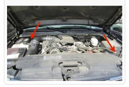
2. Disconnect the MAF sensor wiring and all hose clamps. Then remove your S&B (or OE) intake kit from the truck.
