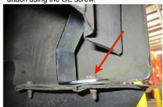
12. Secure the fender liner to the bracket assembly using the screw removed in Step #4
