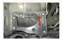
4. Remove the wheel liner support plate by removing 3 fasteners. First remove the screw and fastener from outside the wheel liner. The third fastener can be removed easier from inside the engine compartment located on the inner fender.
