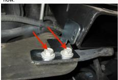
7. Install the 4 Speed nuts (F) by pushing them down until they clip into the holes on the Scoop Inlet (B).
