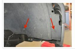
5. Install the Scoop Channel (A) taking the place of the air box mounting tray. Install the 2 OE grommets in the larger holes. Mount up top using the 3 M6x1.0x30mm Screws (E) and 6mm Washers (D).
