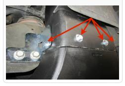
2. Install the four Speed nuts (F) by pushing them down until they clip into the holes on the Scoop Plug (C).
