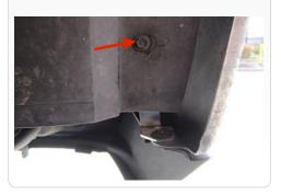
13. Check to make sure the Scoop assembly does not interfere with the wheel or wheel well liner. Turn the wheel in both directions while trying to simulate full suspension travel.
