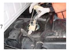
5E-2. Drill a 1-1/8" hole at the selected location in the fuel tank for the suction tube. Hold a container below the drill point to catch debris.
