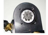
Step 7 Install the gerotor cap. Be very careful to index the cap to position the wide space between the half moon cuts to the bottom.
