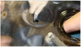
Figure 50 5E-4. Install the grommet in the new suction tube access hole.
