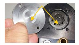
Step 8 Replace the cap into position. Be very careful, do not pinch the O'ring. Torque the cap screws. in an opposing pattern.
