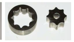
Step 6 Align the teeth and install the outer gear.
