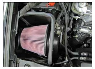
9. Flex the heat shield inward towards the engine then install the K&N<sup>®</sup> air filter onto the filter adapter and secure with the provided hose clamp. Secure the heat shield with two of the remaining factory bolts from step #5.
