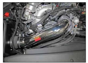
13. Install the K&N<sup>®</sup> intake tube into the coupler installed onto the filter adapter and then into the coupler installed onto the filter inlet. Adjust the tube for best fit and then secure with the provided hose clamps.
