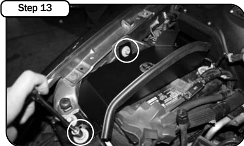
Loosen the 2 bolts near passenger side battery for scoop install using 13mm socket or wrench. Attach trim seal to scoop and align to cut-out on housing. Re-install bolts and tighten. Note: Make sure the positive battery terminal is covered with factory cap.
