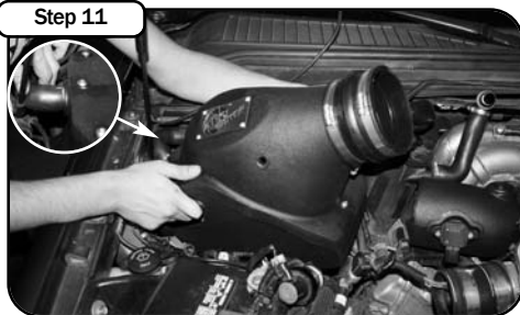
Install intake box into vehicle and position to factory. Make sure intake box sits securely in grommets.
