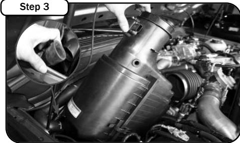
Take auxiliary air line out of air box. Lift and pull firmly then remove OE air box out of vehicle.
