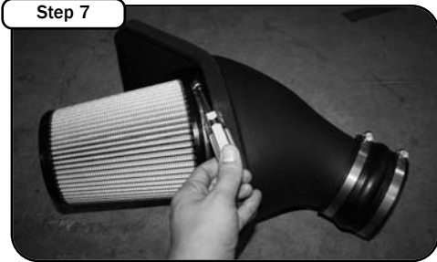
Attach air filter to cover using 5/16" nut driver. Attach hump coupler to end of tube with clamps provided. Do not tighten.
