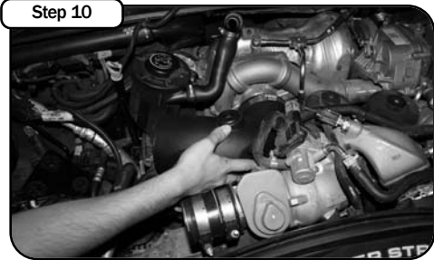
Install new tube into vehicle and position coupler inside of tube on turbo. Note: make sure bead on coupler sits on turbo. The clamp on tube will secure the coupler inside of tube. Do not tighten.
