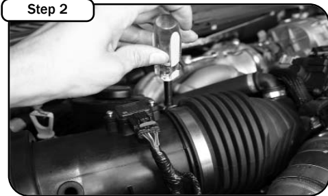
Remove filter minder out of air box. Loosen factory clamp with 5/16" nut driver. Disconnect MAF sensor harness.
