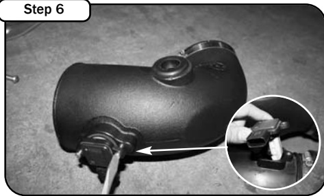
Remove MAF sensor from stock air box using t-20 torx bit provided. Install into new tube using gasket and M4 screws and tighten using flat head screwdriver. Install grommet to hole on tube.
