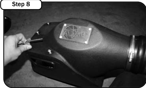
Attach cover to bottom half of new air box and secure using the six 5/16" button head screws provided.
