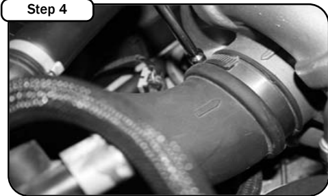
With 5/16" nut driver loosen both clamps on turbo and air box side.
