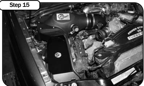
Your installation is now complete. Make sure all hoses and clamps are tight. Check and retighten connections and filter after a few hours of operation. Thank You for choosing aFe! NOTE: Place enclosed CARB EO sticker on or near the air intake system on a smooth/clean surface. EO identification label is required to pass the smog test inspection.
