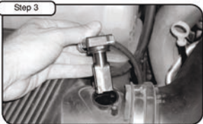
Disconnect MAF sensor harness and remove carefully. Note: MAF sensor can be damaged easily!
