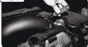
Install 05-01072 tube to turbo side with 05-00033 reducer coupling and clamps provided and position to tube on housing. Do not tighten clamps.
