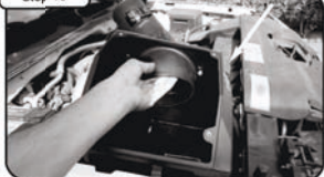
Install housing with tube into vehicle and position.
