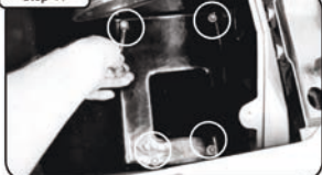
Use the 4 bolts from step 9 and tighten housing using 10mm socket or wrench.
