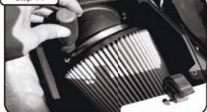
Install air filter and tighten using 5/16" nut driver. Attach cover to housing using provided button head screws. Tighten using 5/32" allen key. Reconnect battery terminals.
