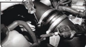
Install hump coupling with clamps provided and secure. Tighten all clamps using 5/16" nut driver. Reconnect MAF sensor harness.
