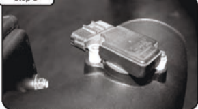
Install MAF sensor into new tube. Use provided screws, nylon spacers and gasket and tighten using phillips screwdriver. Note: Make sure nylon spacers are between sensor and tube.
