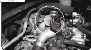
Loosen clamp on turbo with 5/16" nut driver. Remove factory intake tube.
