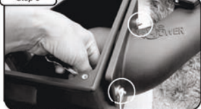
Attach tube to outside of housing using screws, nuts and fender washers provided and tighten using 7/16" socket or wrench.
