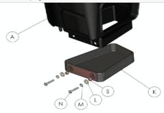
7. Carefully remove the IAT sensor from the stock air box lid. Use the supplied 8-32 Screws
