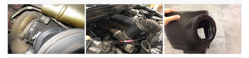
6. (OPTIONAL) For those concerned about minimal engine heat; install the Box Plug (K) onto the bottom of the Air Box (A) using the provided 1/4-20 Screws (N), Lock Washers (M), Flat Washers (L) and Locknuts (S). For those seeking additional air flow, set the box plug aside.
