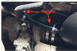
10b. The stop bead on the Intake Tube (B) should be sealed up to the tube seal. Slide the air filter onto the intake tube and tighten the #88 Hose Clamp (S). Align the box prongs on the bottom of the air box with the grommets on the side of battery tray and push down on the box to completely seat the prongs onto the grommet. Tighten the hose clamp at the turbo and CCV line.
