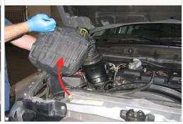
6. Install the Tube Seal (C) onto the Air Box (A).
