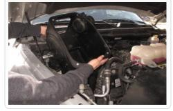
**31.** Install the S&B tube assembly and connect to the factory turbo inlet and tighten the hose clamp.
