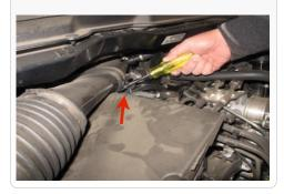
$9. \ {\rm Remove \ the \ air \ box \ lid \ by \ lifting \ up \ and}$ out
