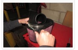
**28.** Install the S&B air box, make sure the bottom grommets align with the factory plastic post underneath.
