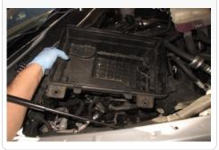
14. Install both grommets on the bottom of the S&B air box.
