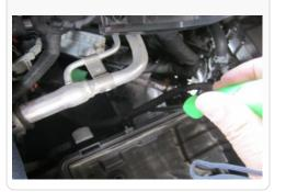
13. Remove the two factory grommets on the bottom of the factory air box.
