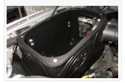
**32.** Slide the coupler towards the S&B air box over the MAF. Tighten down the hose clamp and make sure the tube is aligned properly.
