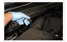
3. Disconnect the MAF sensor harness by
