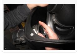
**29.** Use the provided hardware (L&M) to attach the S&B air box to the brackets.
