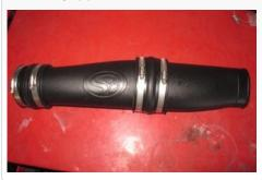
$\begin{array}{l} \textbf{26. Install the Hose Clamp (H) onto the MAF} \\ \textbf{Adapter (B)}. \end{array}$
