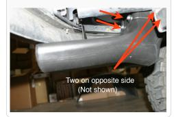
4. From under the truck, remove the two nuts behind the bumper on either side of the frame using a 18mm socket. Slide the mounting brackets off the studs and remove the scoop base.
