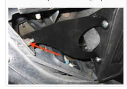
7. Reinstall the two 1/4"-20 screws and washers to the back of the scoop channel. Double check to make sure all hardware is secure and the system is properly positioned.
