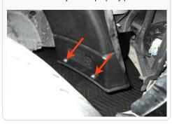
8. Reinstall the wheel well liner using the (8) screws that were removed in step #2. Make sure all of the screws are started before tightening them down.
