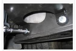
6. Mount the front tab of the "L" bracket to the stud on the bumper using the 18mm nut. Tighten down both 18mm nuts to the back side of the bumper to the OE torque specs.
