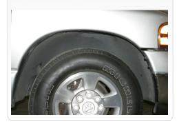
2. Using a pair of pliers, push the pin attaching the wiring harness to the inside. Then remove the wheel well liner from vehicle by pushing it in and then down to remove.
