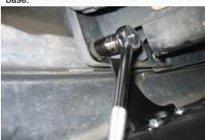
5. Insert the Scoop plug (A) into the scoop channel. Then attach the "L" bracket (B) to the scoop channel using two of the 1/4"-20 screws and washers removed in step #3.
