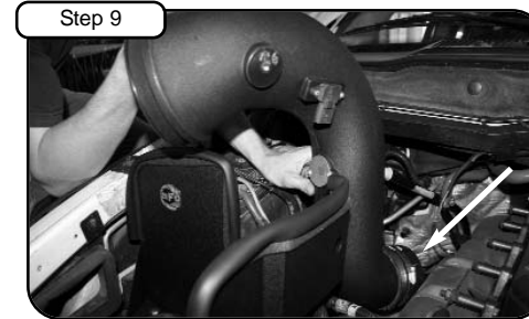
Install hi-temp coupler with clamps provided to tube. Now install tube into vehicle.
