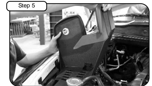
Install 3/4" Trim seal to housing. Now install housing into vehicle.
