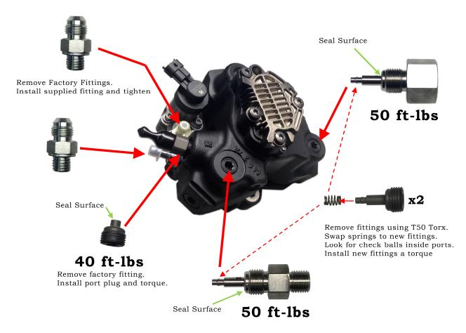
Note: A useful hint for installing the fittings is to install the pump on the pump bracket and clamp the bracket in a vice.
