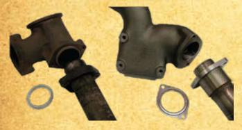
A huge complaint among 7.3L owners is the leaking up-pipe gaskets. The factory donut-style gaskets were originally designed for low pressure exhaust couplings, like those found in most gasoline vehicles. The drive pressure required to drive the turbine wheel in the turbocharger causes the donut gaskets to wear prematurely. The ATS pedestal and up-pipes do not use the donut seal. The ATS system was designed with leak-free stamped sheet metal gaskets.
