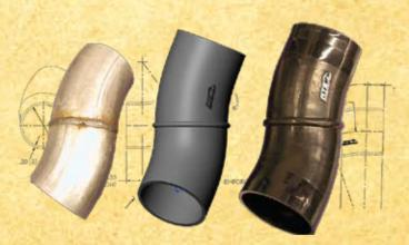
The picture on the left shows the evolution of the intake pipe. From left to right you will see the steel prototype, 3D Model and the final four-inch silicone intake. The Aurora 3000 and 4000 kits include the four inch-intake and the T3 pedestal. The Aurora 5000 and 6000 kits include the five-inch intake and the T4 pedestal. Both intakes are designed to connect directly to the factory crankcase breather coupling.
