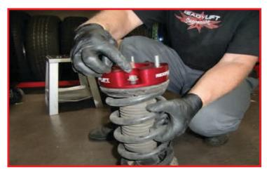
Reattach the strut to the strut tower in the vehicle using provided M10 flange nut. Do not tighten at this time.
