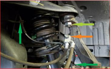
Remove the three upper strut mounting nuts.
