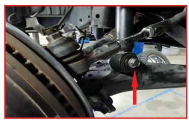
Support the lower control with a suitable jack, With the upper ball joint nut loose, strike the ball joint boss with a dead blow hammer to dislodge the taper (indicated from the red arrow). Once the taper is dislodged remove the upper ball joint hardware, and separate the UCA from the knuckle.
