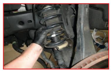
Attach the ReadyLIFT strut extension to the top of strut using the factory hardware to fasten, Torque to 30 ft lbs.
