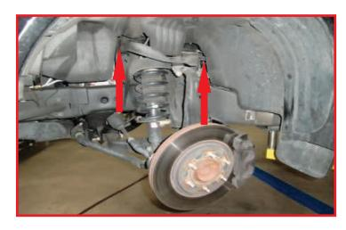
Remove ABS wire from their steel brackets. Remove the brake lines from the knuckle. Remove the cotter pin from the upper ball joint, and loosen but don not remove the ball joint nut.
