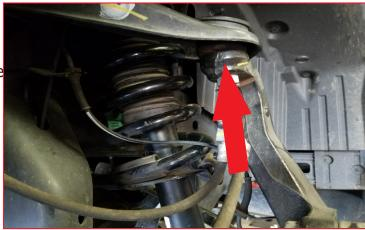
Loosen but do not remove the lower control arm (LCA) hardware at the frame. Lower the LCA while supporting the knuckle and remove the strut from the vehicle. Take care to not over extend or stretch the ABS-rubber brake lines. Adjust as necessary.
