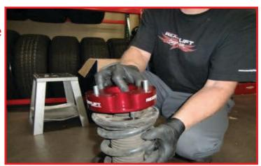
The strut assembly will be clocked 180 degrees for reinstallation.
