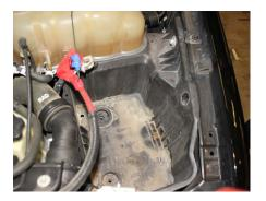
Remove the 2 coolant lines from fuel cooler assembly and remove the fuel line banjo bolts from the top side of the fuel cooler assembly.
