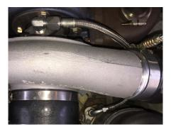
If you will not be using an external wastegate, block the wastegate port on the cast elbow using the supplied plug and clamp.
