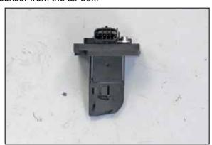
28. Install the mass air sensor into the K&N® mass air sensor adapter and secure with the provided hardware.
