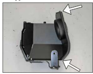
23. Install the provided edge trim onto the heat shield as shown.
