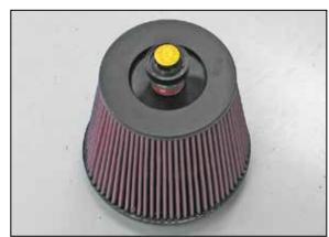
37. Install the filter minder along with the provided grommet into the  $K\&N^{\otimes}$  air filter as shown.
