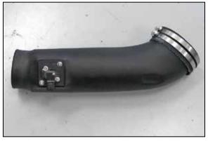
30. Install the provided silicone hose (08540) all the way onto the  $K\&N^{\odot}$  intake tube so the end of the tube is exposed.
