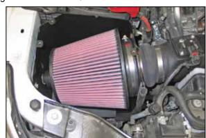
38. Feed the  $K\&N^{\otimes}$  air filter top first into its location, then rotate it back and install onto the filter adapter. Secure the air filter with the provided hose clamp.
