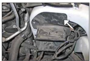
17. Remove the push pin securing the top of the fresh air intake duct.
