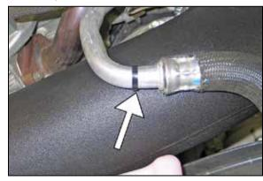
32. Secure the coolant pipe to the insert of the K&N® intake tube with the provided mounting tie wrap
