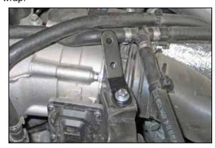
33. Install the coolant hose bracket onto the fan shroud as shown using the provided hardware.
