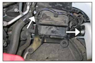
12. Remove the two bolts that secure the air box mounting bracket to the core support and inner fender.
