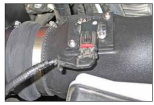
35. Reconnect the mass air sensor electrical connection. Secure the mass air sensor wiring harness to the A/C recharge pipe with the provided tie wrap.
