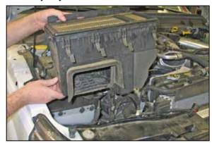
11. Remove the lower air box from the vehicle. NOTE: K&N Engineering, Inc., recommends that customers do not discard factory air intake.
