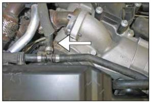
8. Loosen the hose clamp that secures the intake tube to the engine inlet.
