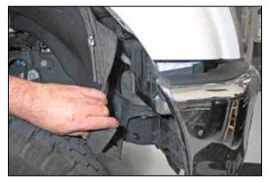
15. Remove the 5 bolts and one push pin securing the front of the inner fender panel and then pull the inner fender panel back to gain access to the bottom of the fresh air intake duct.
