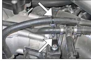
34. Secure the two coolant hoses with the provided mounting tie wraps as shown.
