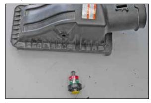
36. Remove the filter minder from the factory upper air box.
