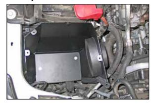
24. Set the heat shield assembly into position and secure with the factory mounting hardware from step #12.
