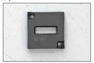
26. Attach the provided gasket onto the mass air sensor adapter as shown.
