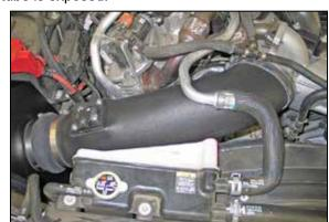
31. Install the intake tube into the silicone hose attached to the filter adapter and align the tube with the factory intake. Slide the silicone hose onto the factory intake and the secure the tube with the hose clamps.
