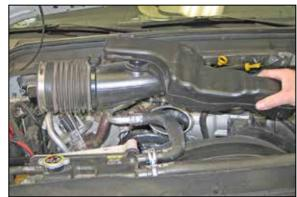
9. Remove the intake tube from the vehicle.
