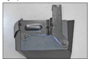
22. Install the factory air box mounting bracket onto the heat shield as shown so that the mount stand-offs installed in step #20 snap into the factory mounting grommets.
