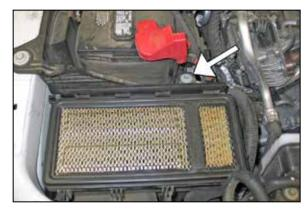
10. Remove the bolt securing the lower air box to the battery tray.
