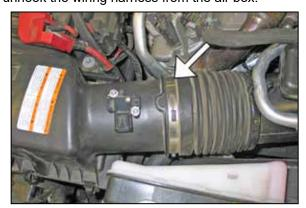
3. Loosen the hose clamp that secures the intake tube to the upper air box.
