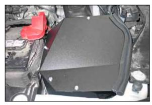
40. Attach the heat shield lid onto the heat shield and secure with the provided hardware.
