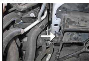
18. Unhook the wiring harness secured to the core support through the fresh air intake duct.
