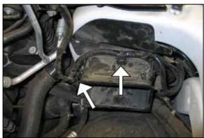
14. Unhook the wiring harness from the fresh air intake duct.
