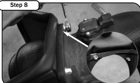
Install trim seal to housing, make sure cutout is at pem-nut on housing. Install tube to outside of housing. Tighten using hex screws, split and flat washers provided with 3/8" socket or wrench.
