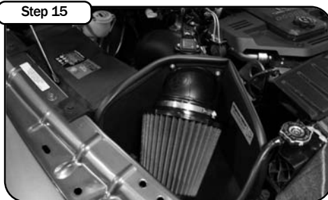
Place the included CARB EO Sticker on or near the intake system on a smooth, clean surface. E.O. identification label is required in passing the Smog Check Inspection. Your installation is now complete. Check all clamps and connections. Periodically check all clamps and hoses. Thank you for choosing aFe!
