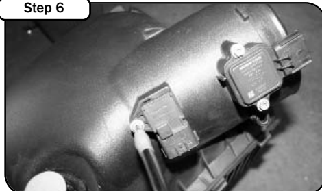
Remove the MAF sensor and the temp sensor with T-20 torx bit provided.
