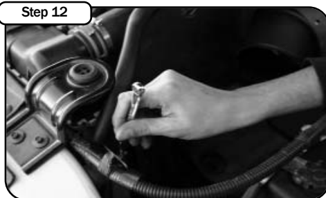
Step 12 Use supplied (M6 nut, two washers) and tighten housing. Two washers are supplied to allow for a washer on both ends of tab if needed
