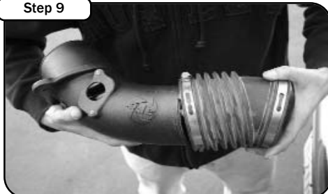
Step 9 Reinstall factory accordion coupler onto tube and install tube into vehicle Do not tighten clamp until final assembly.
