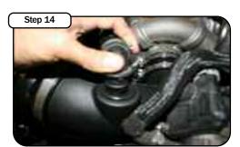
Re-install crank case line into new tube.
