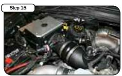
Your installation is now complete. Make sure all hoses and clamps are tight. Check and retighten connections and filter after a few hours of operation. Thank You for choosing aFe! NOTE: Place enclosed CARB EO sticker on or near the air intake on a smooth/clean surface. EO identification label is required to pass the smog test inspection.
