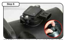
With T-20 torx bit provided loosen the two bolts holding in MAF sensor and remove. Remove grommet for filter minder. With screws and gasket provided, install MAF sensor into new intake tube. (make sure gasket is between sensor and tube) Re-install filter minder grommet into intake tube.
