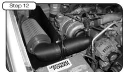
Place the included CARB EO Sticker on or near the intake system on a smooth, clean surface. E.O. identification label is required in passing the Smog Check Inspection.
