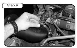
Place crankcase breather elbow onto the nipple of the plastic tube and re-tighten the coupler, be sure to not over-tighten the coupler.
