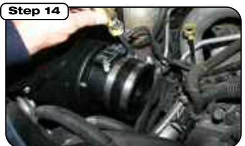
Step 14 Install provided couplers. Be sure to install the small end of the tapered coupler to the turbo inlet housing. The remaining coupler must be installed with the smaller inner diameter attached to the heat shield, and the larger inner diameter will receive the Stage II tube. Install Stage II tube into couplers. Reposition duct clamps if additional clearance is necessary.
