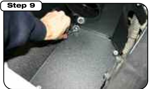
Step 9 Install housing and re-use 4 bolts from step 6. Fasten securely.
