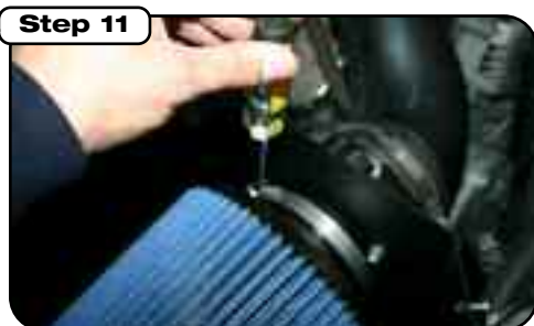
Step 11 Install filter and tighten clamp. Do not use oil or grease.
