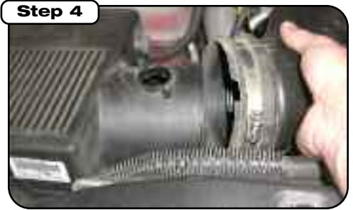
Step 4 Loosen and separate stock intake tube from stock airbox.
