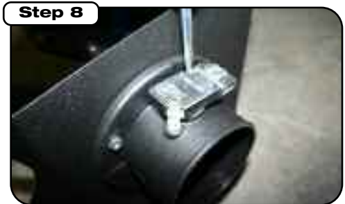
Step 8 Insert mass air flow sensor back into housing and tighten down using 2 screws, 2 nylon spacers and gasket provided between sensor and tube.
