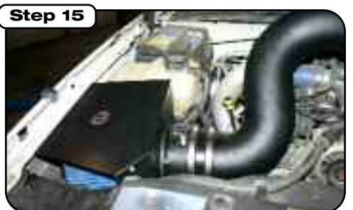
Step 15 Place the included CARB EO Sticker on or near the intake system on a smooth, clean surface. E.O. identification label is required in passing the Smog Check Inspection. Complete Stage 2 kit installed. Make sure all clamps are tight and all components are secure. Check and retighten connections and filter after a few hours of operation.
