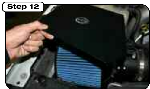
Step 12 Place cover on top of housing and fasten securely using 3 supplied 1/4"-20x3/4 bolts and washers. For stage I kits, make sure all clamps are tight and all components are secure. Check and retighten connections and filter after a few hours of operation. (End of stage 1 installation instructions.)
