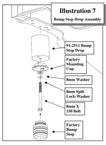
**OE** mounting bolts from the front axle and the rear frame mounting pocket.
