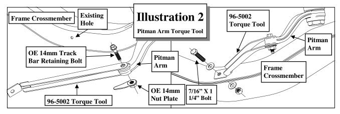
the torque tool will align it's self properly.
