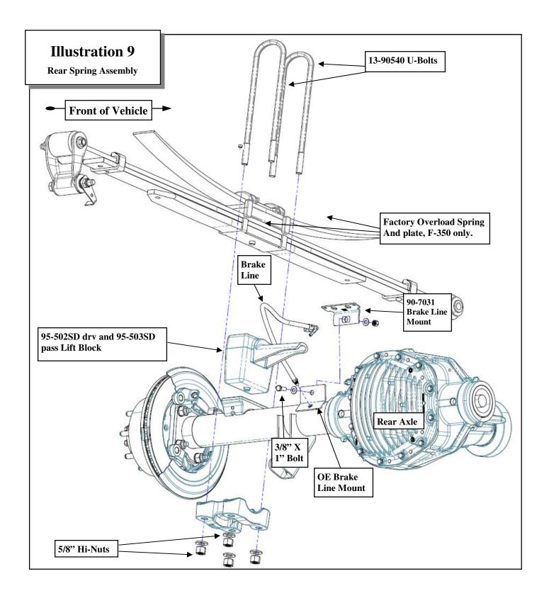
23. On both sides of the vehicle, check the routing of the brake lines and the ABS wire harnesses. There must be no pinching, rubbing, or stretching of either component. Reposition them if needed.
