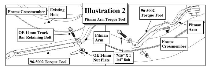
keep the Pitman arm from moving right or left, but allow for movement up the sector shaft. If you do not have this tool, a length of chain or a flat bar with two holes is a suitable replacement.
