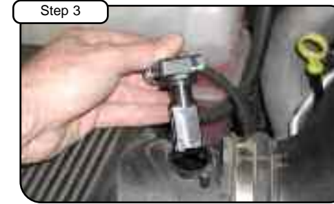
Step 3 Disconnect MAF sensor harness and remove carefully. Note: MAF sensor can be damaged easily!
