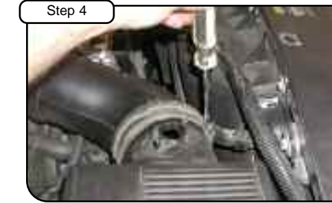
Step 4 Loosen clamp on air box with 5/16" nut driver.
