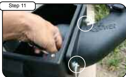
Step 11 Attach tube to outside of housing using screws, nuts and fender washers provided and tighten using 7/16" socket or wrench.
