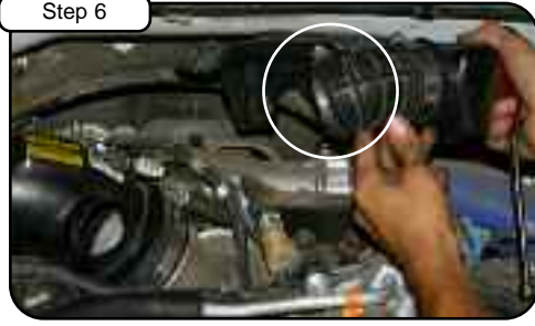
Step 6 Cut clamp on resonator box connected to factory intake tube and pull back. Replace with mini # 040 clamp provided (see step 18). Do not tighten.
