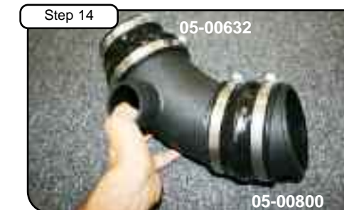
Step 14 Attach reducer coupler (05-00632) to tube with clamps and hump coupler (05-00800) with clamps. Pull back hump coupler for easier installation. Do not tighten.
