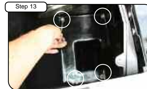
Step 13 Use the 4 bolts from step 9 and tighten housing using 10mm socket or wrench.
