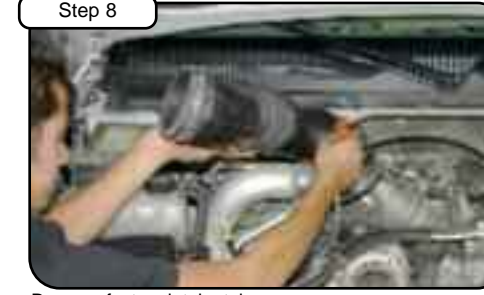
Step 8 Remove factory intake tube.
