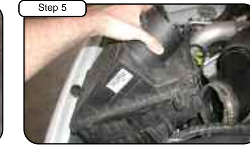
Step 5 Lift and pull air box out of vehicle.
