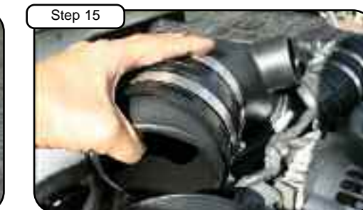
Step 15 Install tube to turbo inlet flange and position. Make sure reducer coupler is on turbo flange. Do not tighten.
