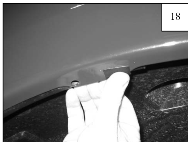
Install Tab (MT1-0014) over existing factory hole.
