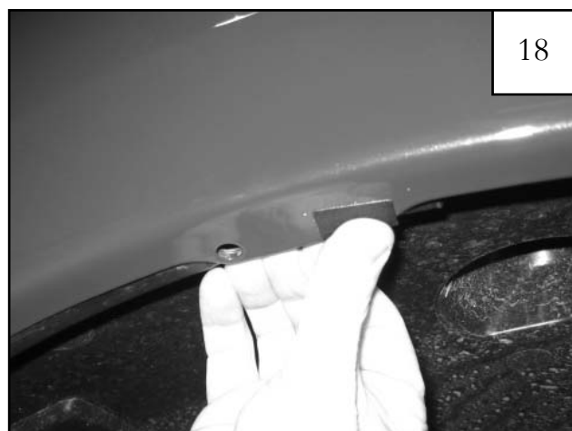
Install Tab (MT1-0014) over existing factory hole.
