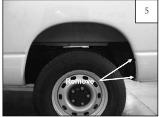
Using an 8mm socket, remove the two factory screws from the rear wheel well. Retain these screws for future use.
