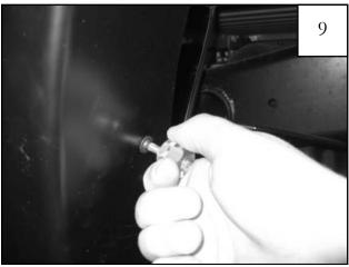
Using a #2 Phillips Screwdriver, insert a supplied Truss Head Screw (SW1-0056) through existing holes in flare and into holes of clips installed in Step 7.
