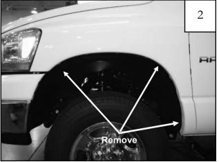
Using an 8mm socket, remove the three factory screws from wheel well. Retain these screws for future use.
