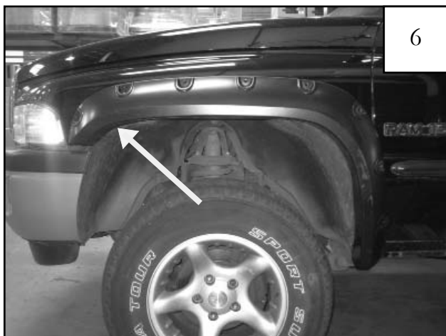
Position flare on fender, pushing flare tightly against fender. Using a right-angle drill with a #2 Phillips bit, drill one supplied Screw (SW1-0066) through plastic of fender flare and into sheet metal of fender using the indents in the flare as a guide.
