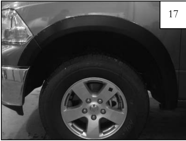
METAL BUMPER ONLY: Completed front flare installation.
