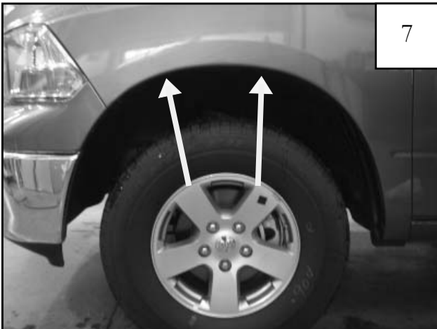
Install #10 U-Clips at these locations. See step 9. NOTE: There are two factory holes near the rearward arrow. The correct hole for install is the one more toward the front of the vehicle.
