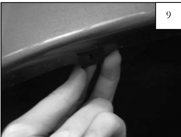
Install #10 U-Clip over existing factory holes.
