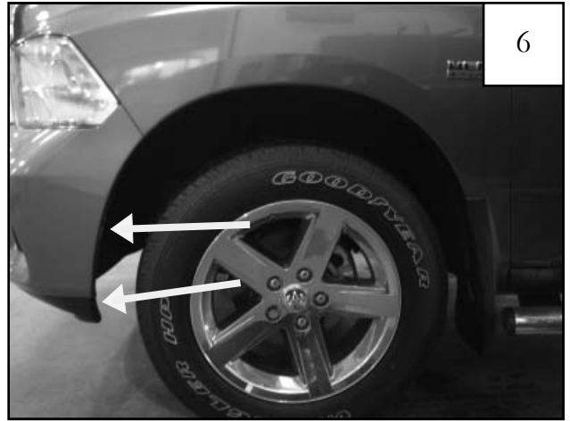
PLASTIC BUMPER ONLY: Remove two factory installed tuflocks.
