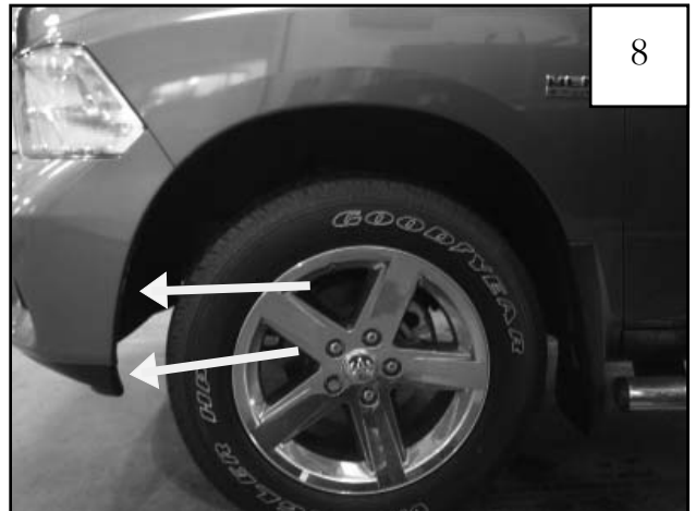
PLASTIC BUMPER ONLY: Install #10 U-Clips at these locations. See step 9.
