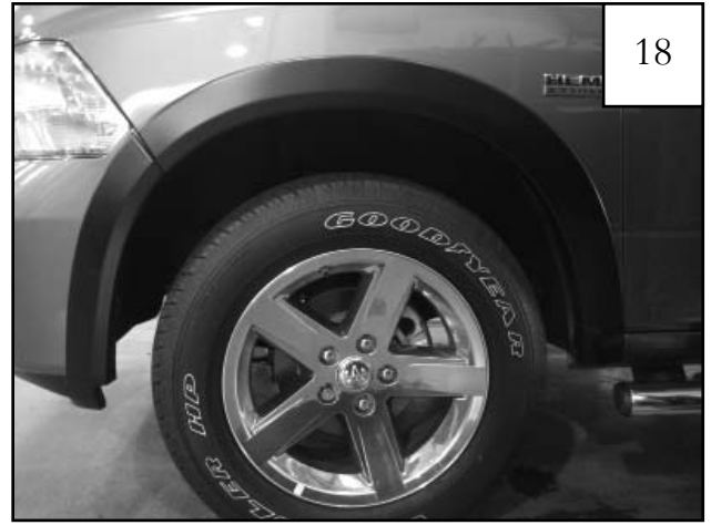
PLASTIC BUMPER ONLY: Completed front flare installation.
