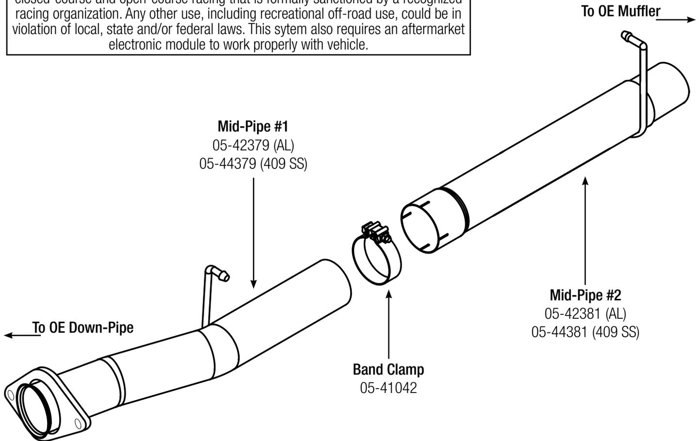
**Step 1: (Read Instructions prior to installation)** Disconnect sensors at the connections. Take caution as not to damage any sensors. Remove CAT/DPF section of your trucks exhaust working your way forward. Take caution not to damage the factory isolation mounts as they will be reused. **It is recommended to not fully tighten the clamps until the entire system has been installed.**
