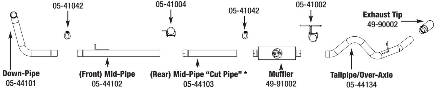
**1: (Read Instructions prior to installation)** Remove your stock exhaust from the rear of your truck working your way forward. Take caution not to damage the factory isolation mounts. If you want to remove the OE downpipe in one piece or without cutting, you must remove the transmission cross member and disconnect the dip-stick tube & sway bar end links. *It is recommended to not fully tighten the clamps until the entire system has been installed.*
