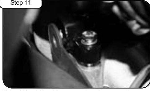
Step 11 Using M6 x 1.00 x 25 screw and washer secure last remaining manifold mount and tighten. Tighten all screws and nuts using 10mm socket or wrench. See Notes 2 & 5.
