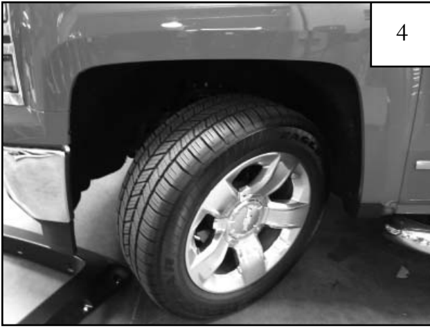
Turn front tire outward for easier installation.
