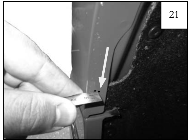
Remove the flare. At the marked locations made in Step 18, measure inward 22mm from the edge of the fender. These are the marks to be drilled.
