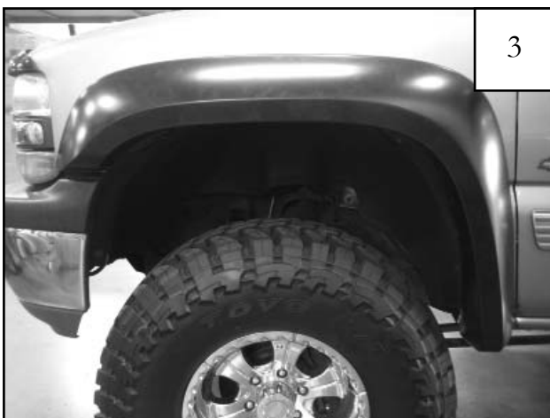
Completed front flare installation.
