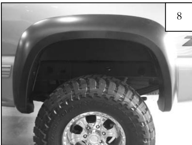
Completed rear flare installation.
